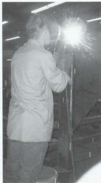
Spending many hours of work on the 20 ft. lowboy, Cory Burns welds gussets to brace the tongue of the trailer.
