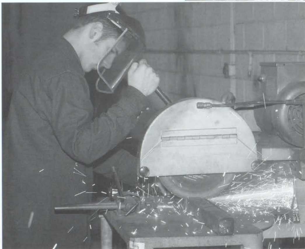
Building a swing for the ag auction in April, Aaron Downs smooths rough places on metal with a grinder.
